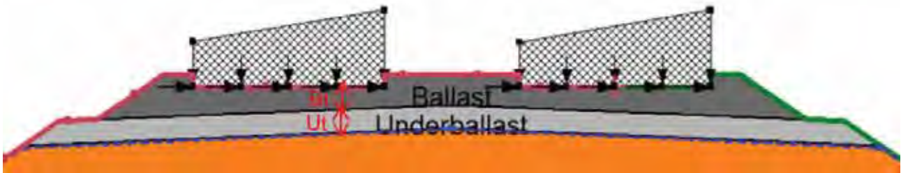
Figur 6: Princip for modellering af sporkasse i SLOPE/W
