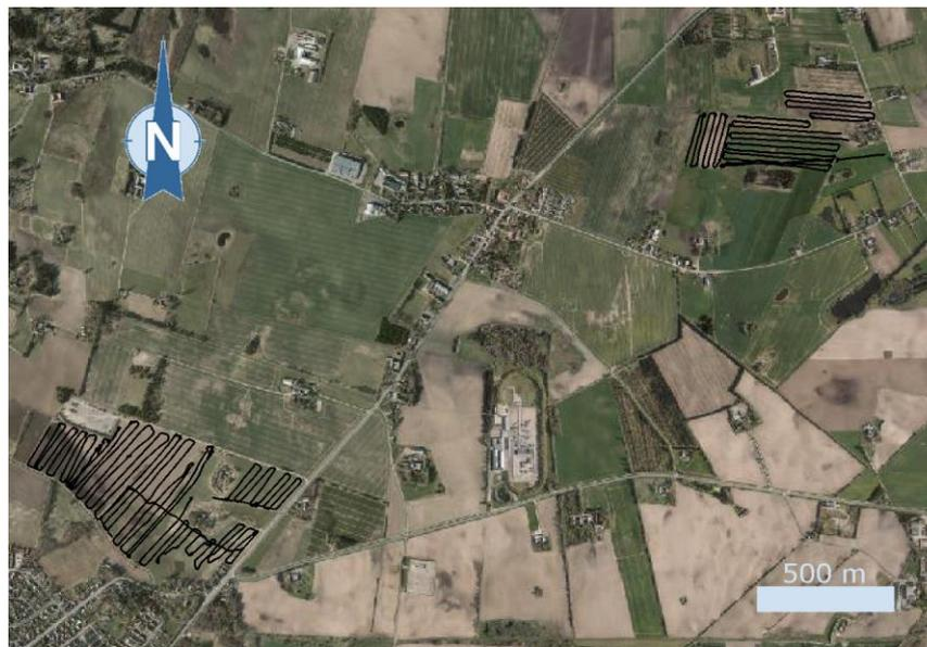
Figure 1. Survey area, with tTEM lines in black. The model spacing along the lines is ~10 m.
